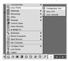
You can also access the Linux Printer Configuration window by typing in "**linux-config**" from the Terminal screen.
